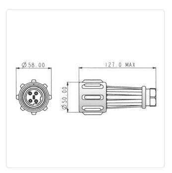
Amperage [A]: 32 Color: Black Protection Code: IP68 Weight: 145.5g Conformities:
