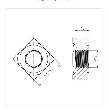
AF / OD [mm]: **DIN928** DIN/ISO: Finish: Plain 9.5 Height [mm]: Material: Steel Material Group: Steel Thread Size: M12
