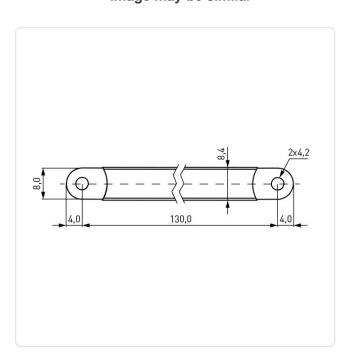
Insulation: Polyolefin 138 Length [mm]: Material: Copper Material Group: Copper Mounting Hole [mm]: 4.2
