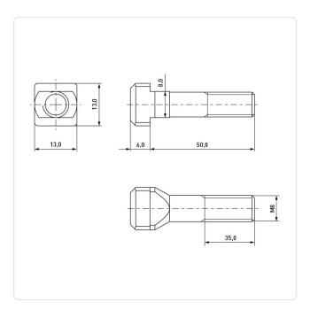
DIN/ISO: **DIN787** Plain Finish: Head Height [mm]:
