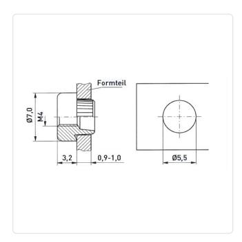
Finish: Plain Height [mm]: 3.2 Material: Steel Material Group: Steel Outer Diameter [mm]: 7 Panel Hole Ø [mm]: 5.5 Panel Thickness [mm]: 0,9 - 1,0 Thread Size: M4 Weight: 0.72g
