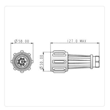
Amperage [A]: 32 Color: Black Protection Code: IP68 Weight: 151g Conformities:
