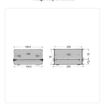
Color: Black Height [mm]: 67 Length [mm]: 220 Material: Steel Material Group: Stahl Width [mm]: 136.5 Weight: 961g Conformities:
