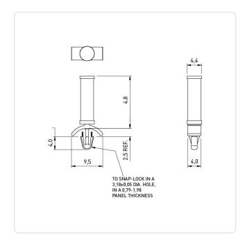
Color: Natural Flammability Class: UL94-V2 4.8 Length [mm]: Material: PA 6.6 Material Group: **Plastic** Panel Hole Ø [mm]: 3.2 Panel Thickness [mm]: 0,8-2,0
