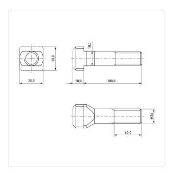
DIN/ISO: **DIN787** Plain Finish: Head Height [mm]:
