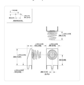
Battery Type: AA-Mignon Finish: Tin-Plated Steel Material: Material Group: Steel Weight: 0.97g
