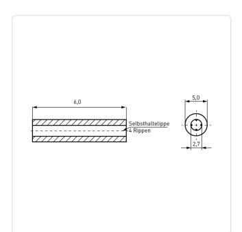
Color: Black Flammability Class: UL94-V2 For Thread Size: M2.5 Inner Diameter [mm]: 2.7 Length [mm]: 6 Material: PA 6.6
