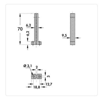
Color: Gray Dist. Mounting Holes [mm]: 12.7 Flammability Class: UL94-V0 Length [mm]: 70
