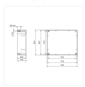
Color: Gray Flammability Class: UL94-HB Height [mm]: 21.8 74 Length [mm]: PA 6.0 Material:
