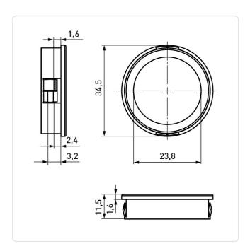
Color: Black Inner Diameter [mm]: 24 Material: PA 6.6 Material Group: Plastic Max. Panel Thickness [mm]: 3.2 Mounting Hole [mm]: 32 Weight: 3.06g Conformities:
