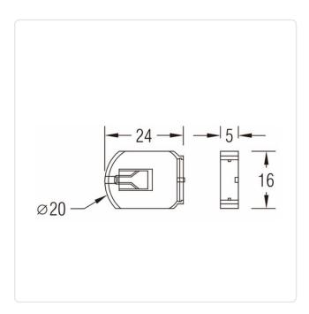
Battery Type: Cell Dia. 20mm
