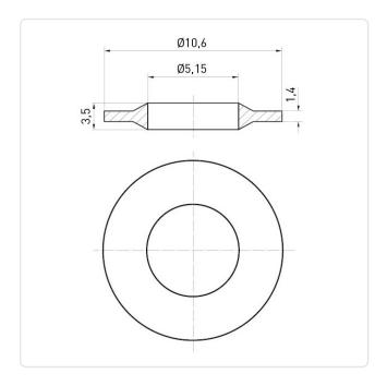
For Thread Size: M5 3.5 Height [mm]: Inner Diameter [mm]: 5.15 Material: PA 6.0 Material Group: **Plastic** Outer Diameter [mm]: 10.6 Weight: 0.12g
