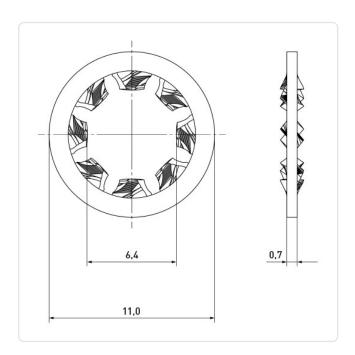
DIN/ISO: DIN6798I Finish: Plain For Thread Size: M6 Inner Diameter [mm]: 6.4
