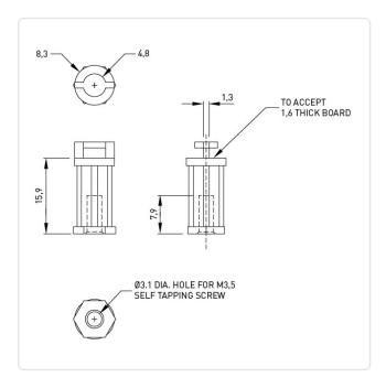
Color: Natural Flammability Class: UL94-V2 Length [mm]: 15.9 Material: PA 6.6 Material Group: **Plastic** PCB Hole Ø [mm]: 3.1 PCB Thickness [mm]: 1,6 Thread Size: M3.5 Weight: 0.54g
