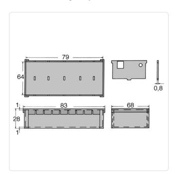
Height [mm]: 28 Length [mm]: 83 Material: Steel Material Group: Stahl
