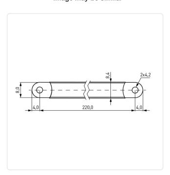
Insulation: Polyolefin 228 Length [mm]: Material: Copper
