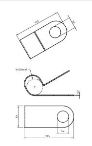
Bundle Diameter [mm]: 5,4 Distance Middle/Middle [mm]: 9.8 Length [mm]: 18.5 Material: Stainless Steel AISI 304 / A2 Stainless Steel Material Group: 3.2 Mounting Hole [mm]: Thickness [mm]: 0.3 Width [mm]: 8.6 Weight: 0.78g Conformities: Reach RoHS SVHC
