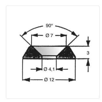
Color: Black For Thread Size: M4 Height [mm]: Inner Diameter [mm]: 4.1 Material: PA 6.6 Material Group: Plastic Outer Diameter [mm]: 12 Weight: 0.24g
