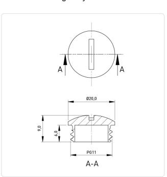
Height [mm]: Material: **Brass** Material Group: Brass Model: Plug Screw Thread Size: PG11
