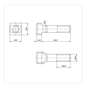
DIN/ISO: **DIN787** Plain Finish: Head Height [mm]: 16
