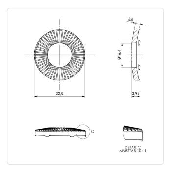
Plain Finish: For Thread Size: M16 Height [mm]: 2.5 Inner Diameter [mm]: 16.4
