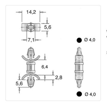
Color: Natural Flammability Class: UL94-V2 Length [mm]: 6.4 Material: PA 6.6 Material Group: **Plastic** PCB Hole Ø [mm]: PCB Thickness [mm]: 0,8-2,0 Panel Hole Ø [mm]:
