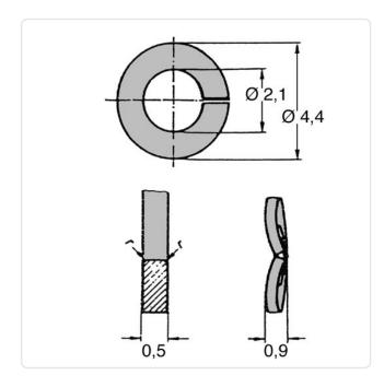
DIN/ISO: DIN128A Finish: Plain For Thread Size: M2 0.5 Height [mm]: Inner Diameter [mm]: 2.1
