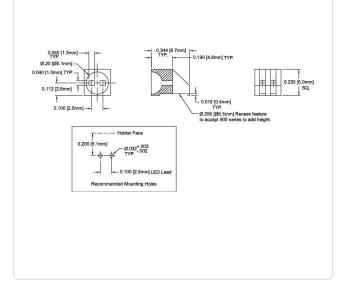
Color:BlackDiameter [mm]:6LED Size [mm]:Ø 5Material:PA 6.0Material Group:PlasticWidth [mm]:6Weight:0.2gConformities:ReachReachROHSCOMPLIANTCOMPLIANT
