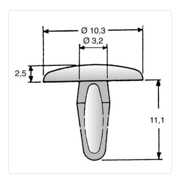
Color: Natural Flammability Class: UL94-V2 Head Diameter [mm]: 10.3 Material: PA 6.6 Material Group: **Plastic** Mounting Hole [mm]: 3.5
