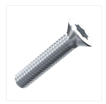
Torx T20 Actuator Size: DIN/ISO: ISO14581 Drive Type: **TORX** Plain Finish: Head Diameter [mm]: 8.4 Head Height [mm]: 2.7
