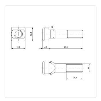
DIN/ISO: **DIN787** Plain Finish: Head Height [mm]:
