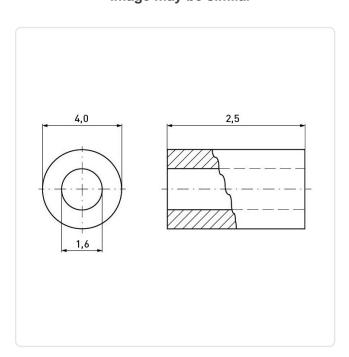
Color: White Flammability Class: UL94-V2 For Thread Size: M1 Inner Diameter [mm]: 1.6 Length [mm]: 2.5 Material: PA 6.0 Material Group: Plastic Outer Diameter [mm]: 4 Weight: 0.05g
