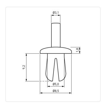
Color: Black UL94-V2 Flammability Class: Head Diameter [mm]: 8.5 Head Height [mm]: 1.8 Length [mm]: 9.2 Mandrel Diameter [mm]: 3.1 PA 6.6 Material:
