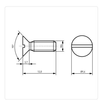
Color: Natural Drive Type: Slotted Head Diameter [mm]: 9.4 Head Height [mm]: 3.7
