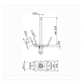
Bending Angle [°]: 25 Finish: Plain Material: **Brass** Material Group: **Brass** Mounting Hole [mm]: 5.2 Panel Thickness [mm]: 0,6-2,0 Plug-In Length [mm]: 7.8 Size [mm]: 6.3x0.8 Tabs: 2 Weight: 3.65g Conformities:
