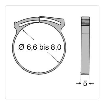
Color: Black UL94-V2 Flammability Class: Material: PA 6.6 Material Group: Plastic Panel Thickness Range [mm]: 6,6-8,0 1.8 Thickness [mm]: Width [mm]: 5 Weight:
