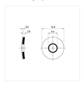
Plain Finish: For Thread Size: M8 Height [mm]: Inner Diameter [mm]: 8.4
