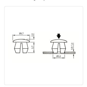
Color: Natural Inner Diameter [mm]: 4.8 Material: PA 6.6 Material Group: Plastic Model: Hole Plug
