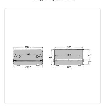
Color: Blue Height [mm]: 67 Length [mm]: 220 Material: Steel Material Group: Stahl Width [mm]: 208.5 Weight: 1049g
