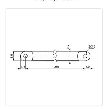
Insulation: Polyolefin 108 Length [mm]: Material: Copper Material Group: Copper
