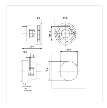
Cable diameter [mm]: Ø 7,5-8,5 Color: Natural Diameter [mm]: 25 PA 6.6 Material: Max. Panel Thickness [mm]: 3 Mounting Hole [mm]: 22
