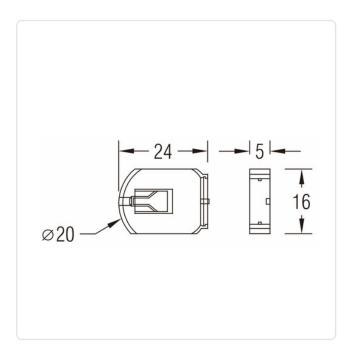
Battery Type: Cell Dia. 20mm
