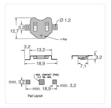
Battery Type: Cell Dia. 12mm
