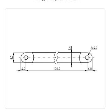
Insulation: Polyolefin 108 Length [mm]: Material: Copper Material Group: Copper Mounting Hole [mm]: 4.2
