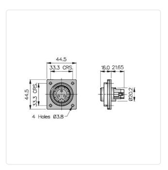
Amperage [A]: Color: Black Protection Code: IP68 Weight: 33g
