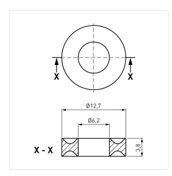
For Thread Size: M6 3.8 Height [mm]: Inner Diameter [mm]: 6.2 Material: PA 6.0 Material Group: **Plastic** Outer Diameter [mm]: 12.7 Weight: 0.26g
