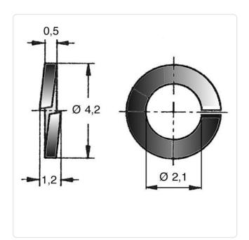
DIN/ISO: DIN127B Finish: Plain For Thread Size: M2 0.5 Height [mm]: Inner Diameter [mm]: 2.1
