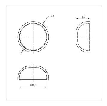
Color: Gray Head Height [mm]: 5.9 Inner Diameter [mm]: 10.8 Material: PA 6.0 Material Group: **Plastic**
