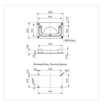
Dist. Mounting Holes [mm]: 94 Height [mm]: 63.5 Material: Steel Material Group: Stahl
