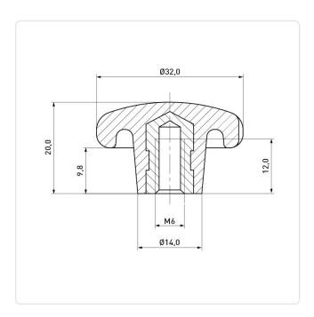
Color: Black Diameter [mm]: 32 Height [mm]: Material: Plastic Material Group: Plastic Thread Size: M6 Weight: 10.46g
